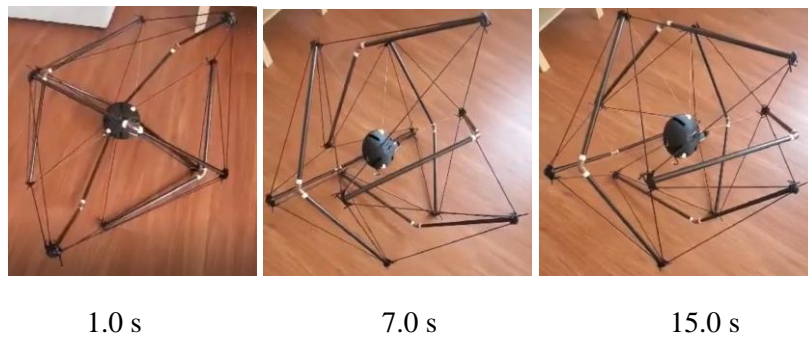
Figure 35: Recentering during Successive Motion, Enclosed 6 Motor Configuration
