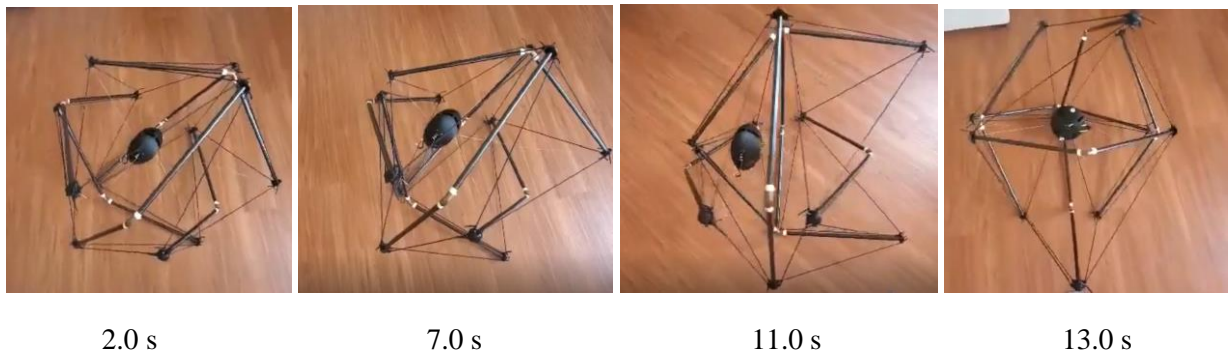
Figure 34: Stage 1 Successive Motion, Enclosed 6 Motor Configuration
