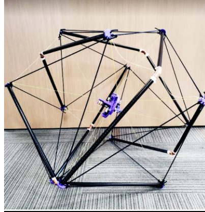
Figure 29: Flounder, 6 Motor Configuration (Updated End Caps not Pictured)
