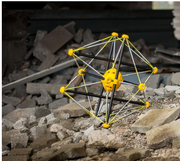
Figure 1: Squishy Robotics' Tensegrity Robot
